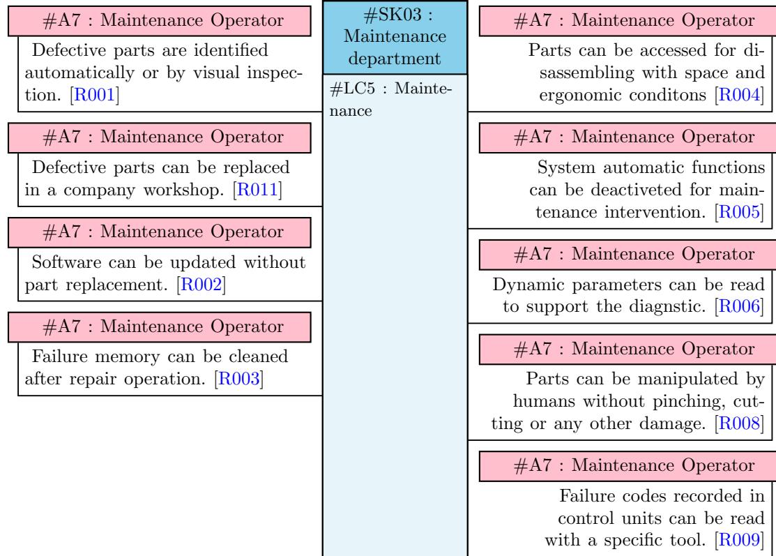
A product has to be maintained and sometimes repaired. Maintenance constraints ensure that these operations can be carried out in good conditions at affordable cost. This block diagram gives an example of maintenance constraints. External elements are repr
