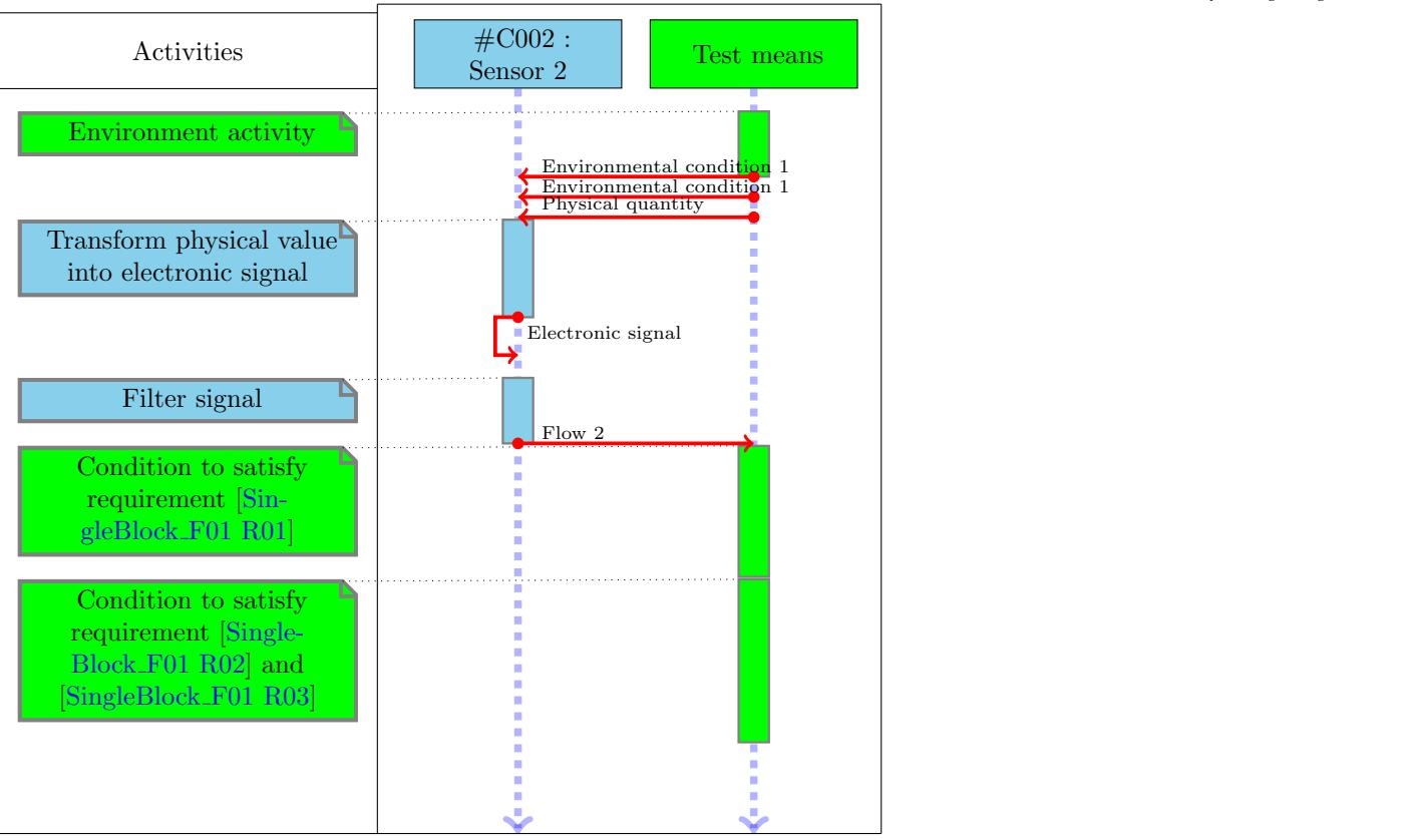
A physical sequence describes a scenario in which the system is split into components.
