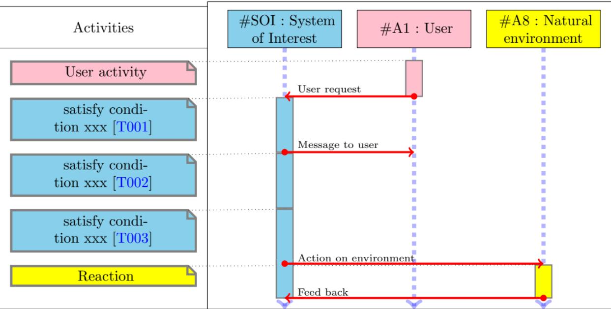
An operational sequence describes a scenario in which the system of interest (SOI) is considered as a whole, without details of the inner components. Only interactions with the external environment (user, external people, physical environment) is describe
