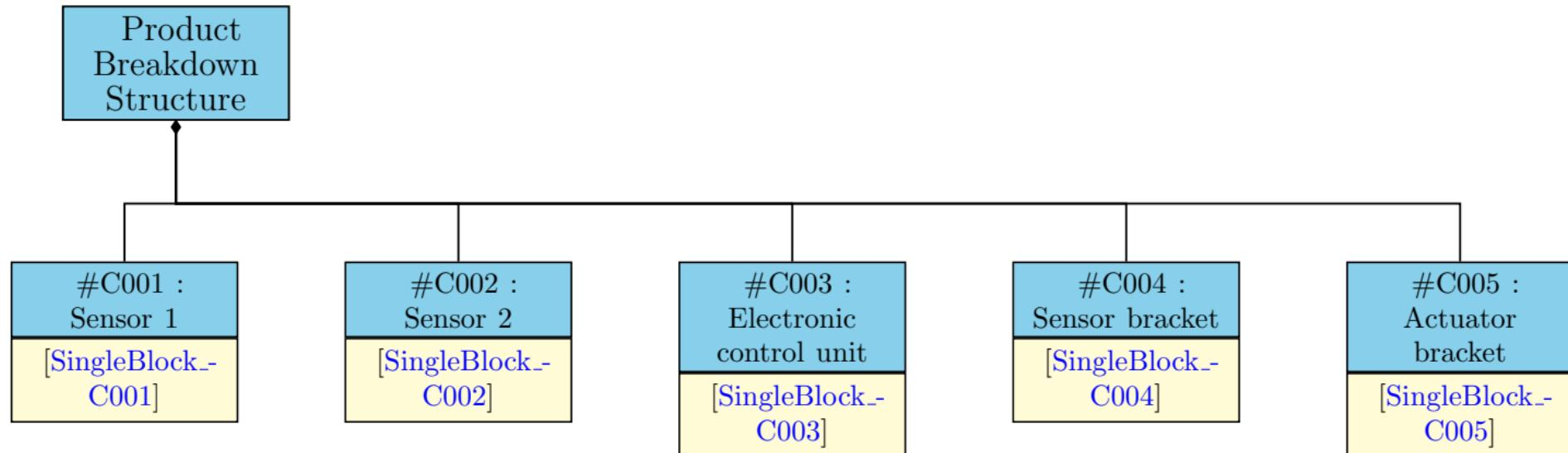
The Product Breakdown Structure contains all the components defined for the system. Detailed description of components and related functional allocations can be accessed via the link in the box compartment.
