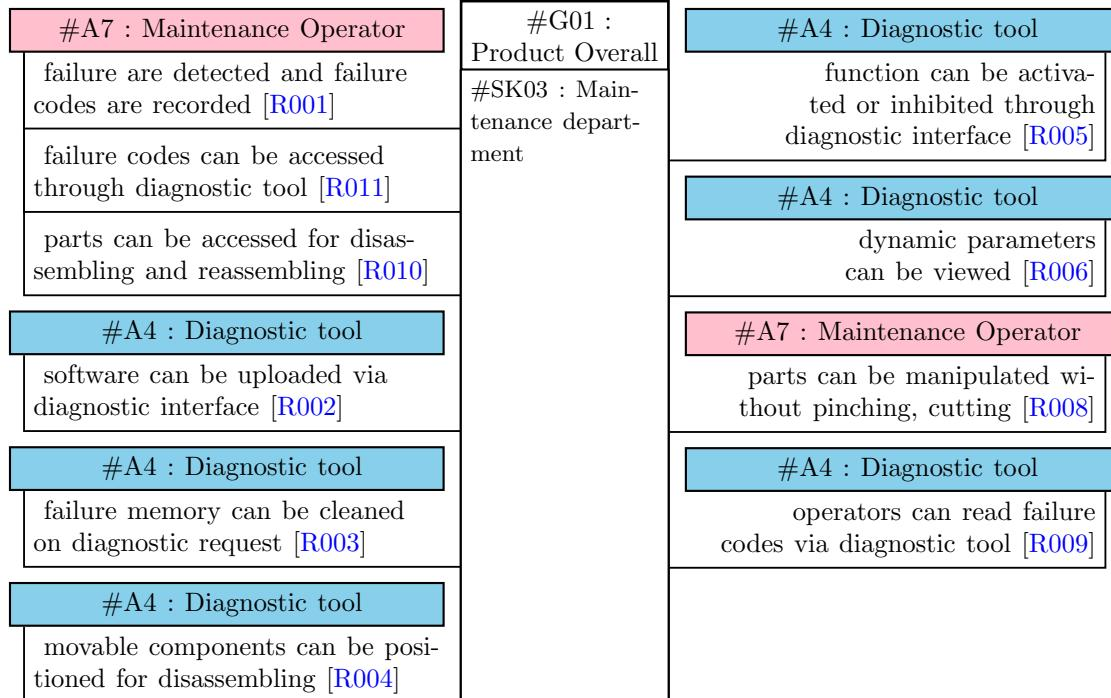
A product has to be maintained and sometimes repaired. Maintenance constraints ensure that these operations can be carried out in good conditions at affordable cost. This block diagram gives a example of maintenance constraints. External elements are represented in lateral boxes and corresponding needs are displayed in a compartment of the box . Text above lines describes the way the system satisfies the need. Hypertext links point to system requirements.
