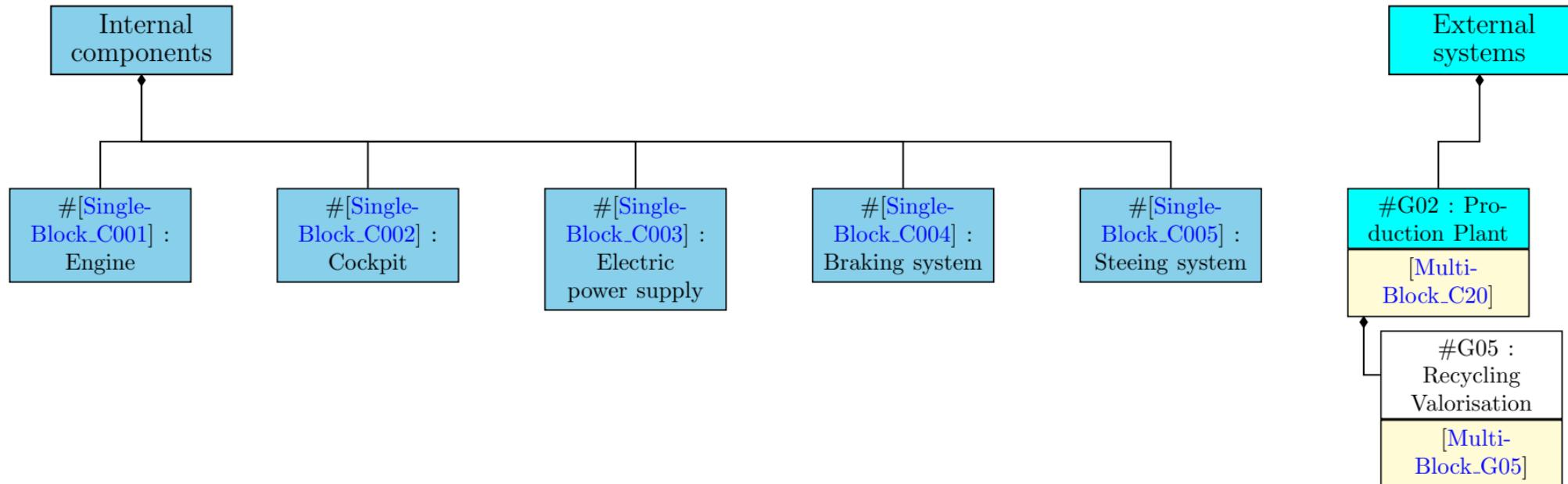
The Product Breakdown Structure contains the components defined for the system. Detailed description of components and related functional allocations can be accessed via the link in the box compartment.
